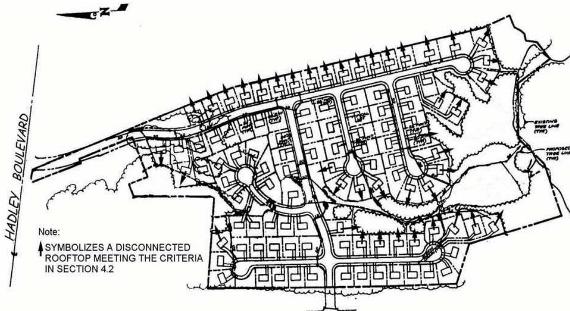
Figure B.2 Schematic of Rooftop Disconnection Credit
