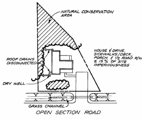
Figure B.5 Schematic of Environmentally Sensitive Rural Development Credit
